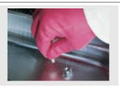
Place the moisturing nozzle in the descaling liquid and allow it to react (moisturing nozzle must be free of scale)
