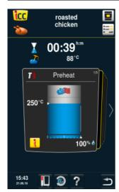
You can open the iCC cockpit by pressing the iCC cockpit button or it will open automatically after 10 seconds.
