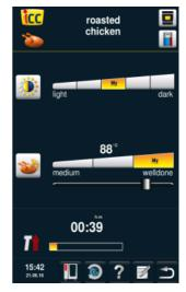
For example, select the browning level (light, dark) and the core temperature/cooking state (rare, welldone).
